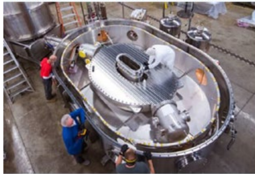
The HTS Magnet was successfully tested up to 20 Tesla at the MIT
